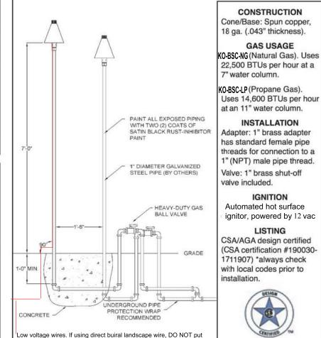
wire directly in concrete. We recommend you protect the wire with PVC, please contact Koahi Systems for more detailed installation instructions.
